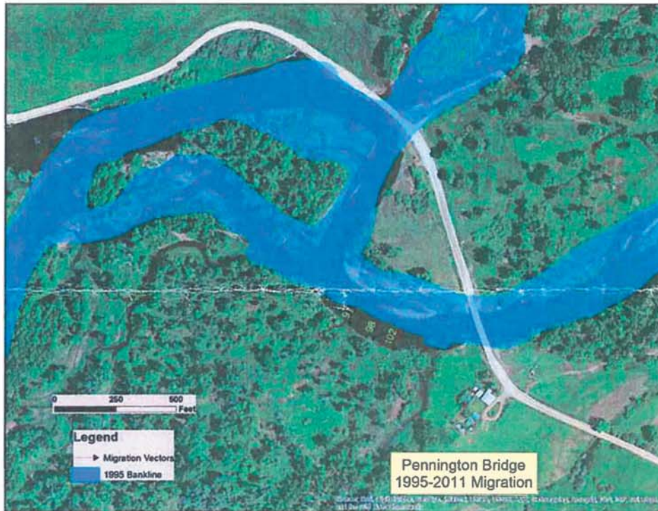
Figure 3. 1995 banklines on 2011 air photo showing ~100 feet of channel migration over 16 years.
